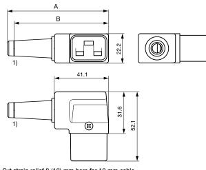
1) Cut strain relief 8 (10) mm here for 10 mm cable A: Strain relief 8 mm: 76.1 mm
